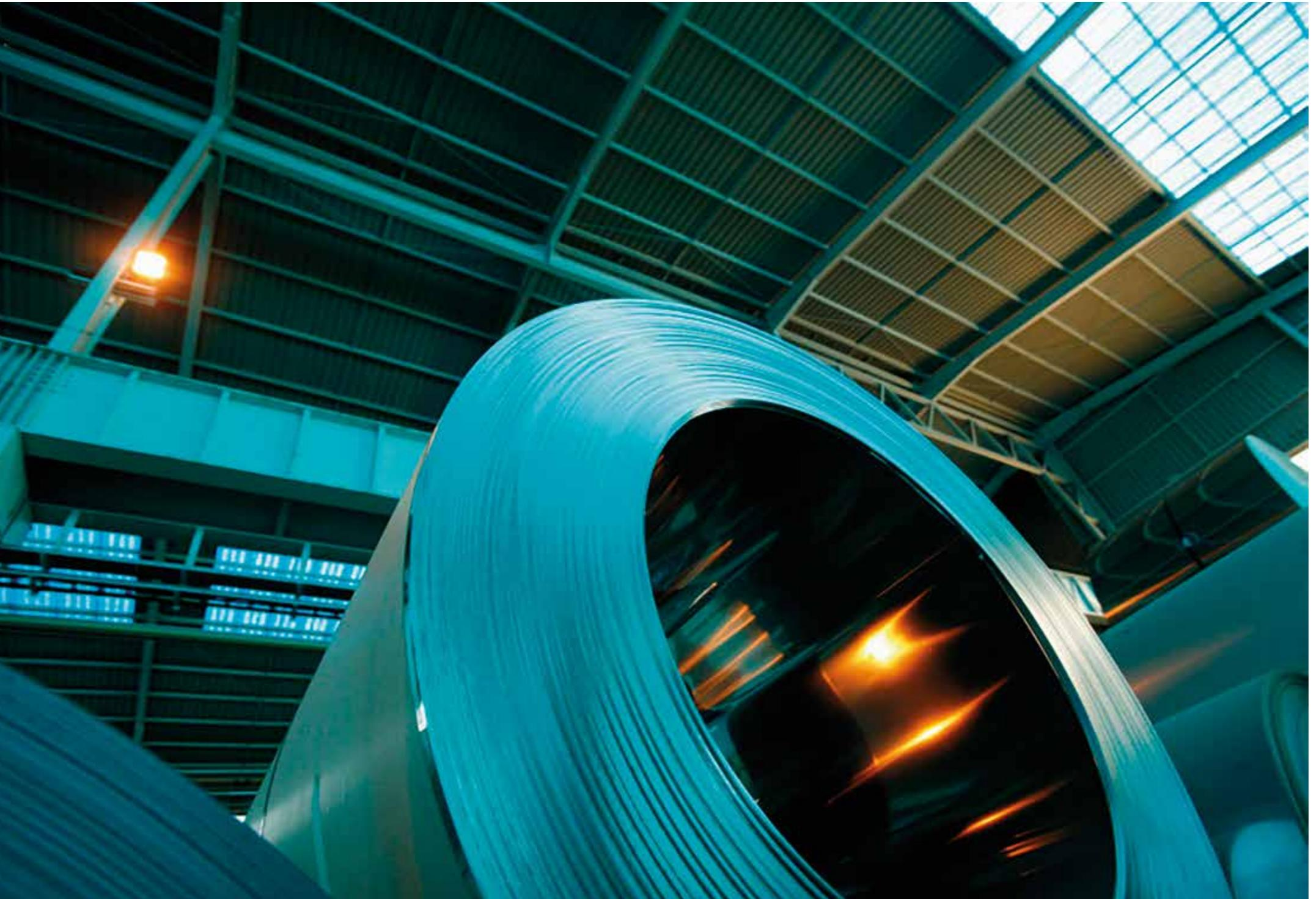
Materials that need to be of greater beauty require a mirror-like finish, which is obtained by means of a thermal treatment in reducing atmosphere ovens (hydrogen): since oxide is not generated on the surface, final treatment makes it possible to give the material a characteristic shine and finish.
