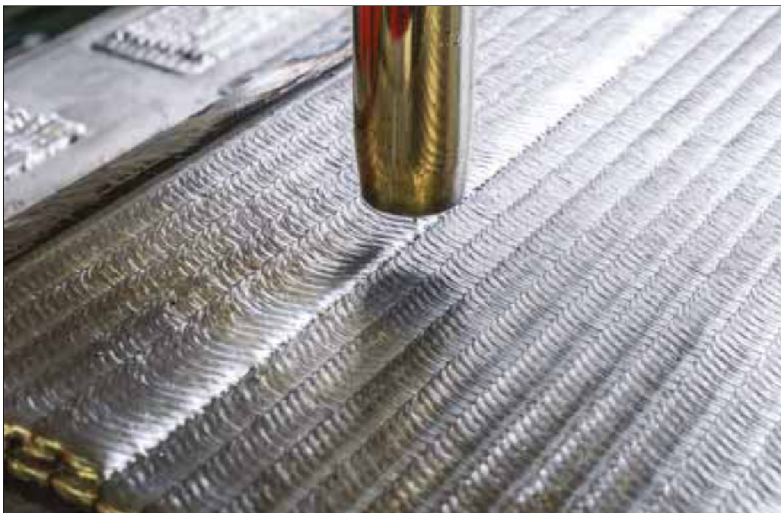
Coating carried out in the Welding Centre of Excellence at VDM Metals.
