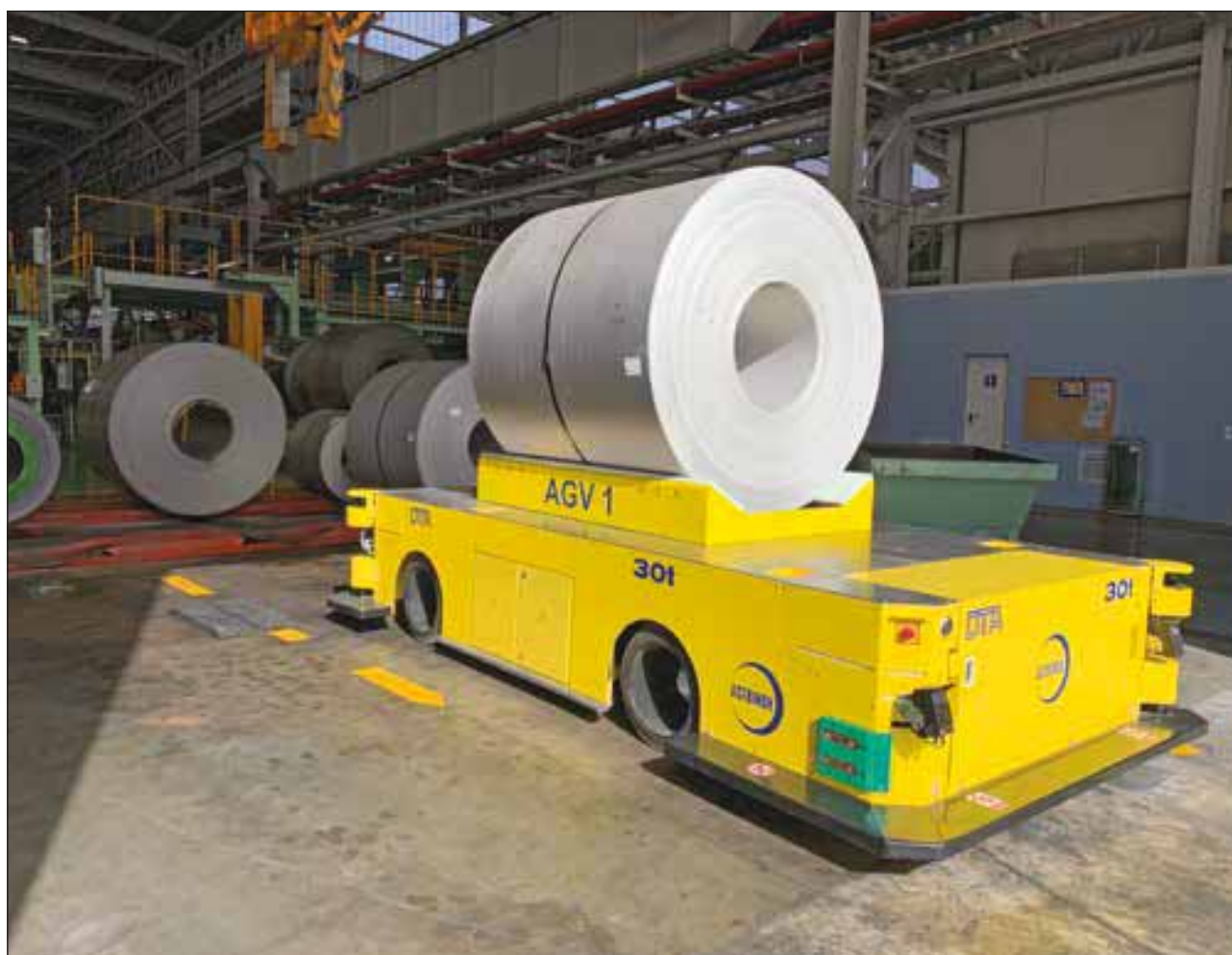
Autonomous Guided Vehicle in the Acerinox Europa Factory.
