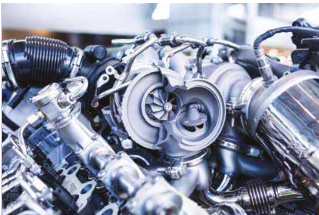
VDM Metals high performance alloys used in turbochargers thanks to their heat resistance.
