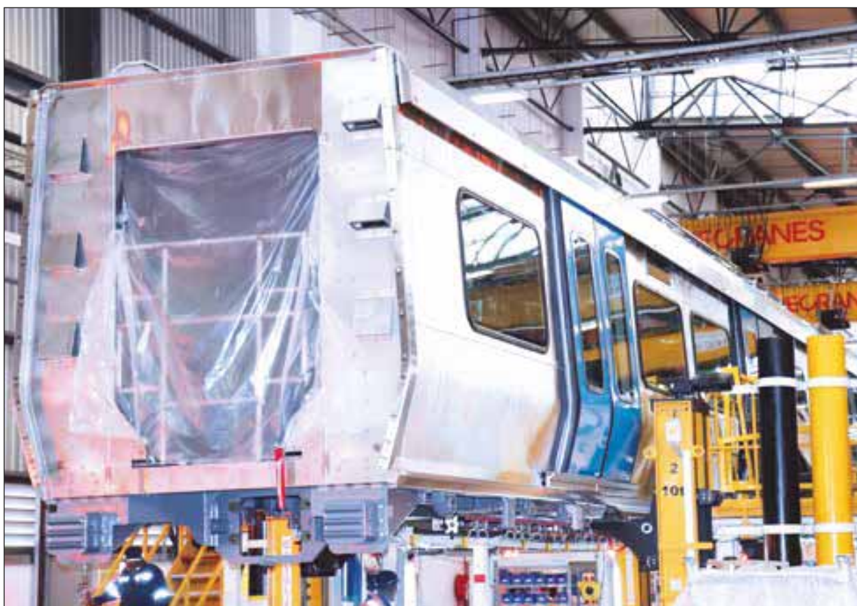
Construction of suburban trains in South Africa with Aisi 301 stainless steel, supplied by the Columbus Stainless Plant
