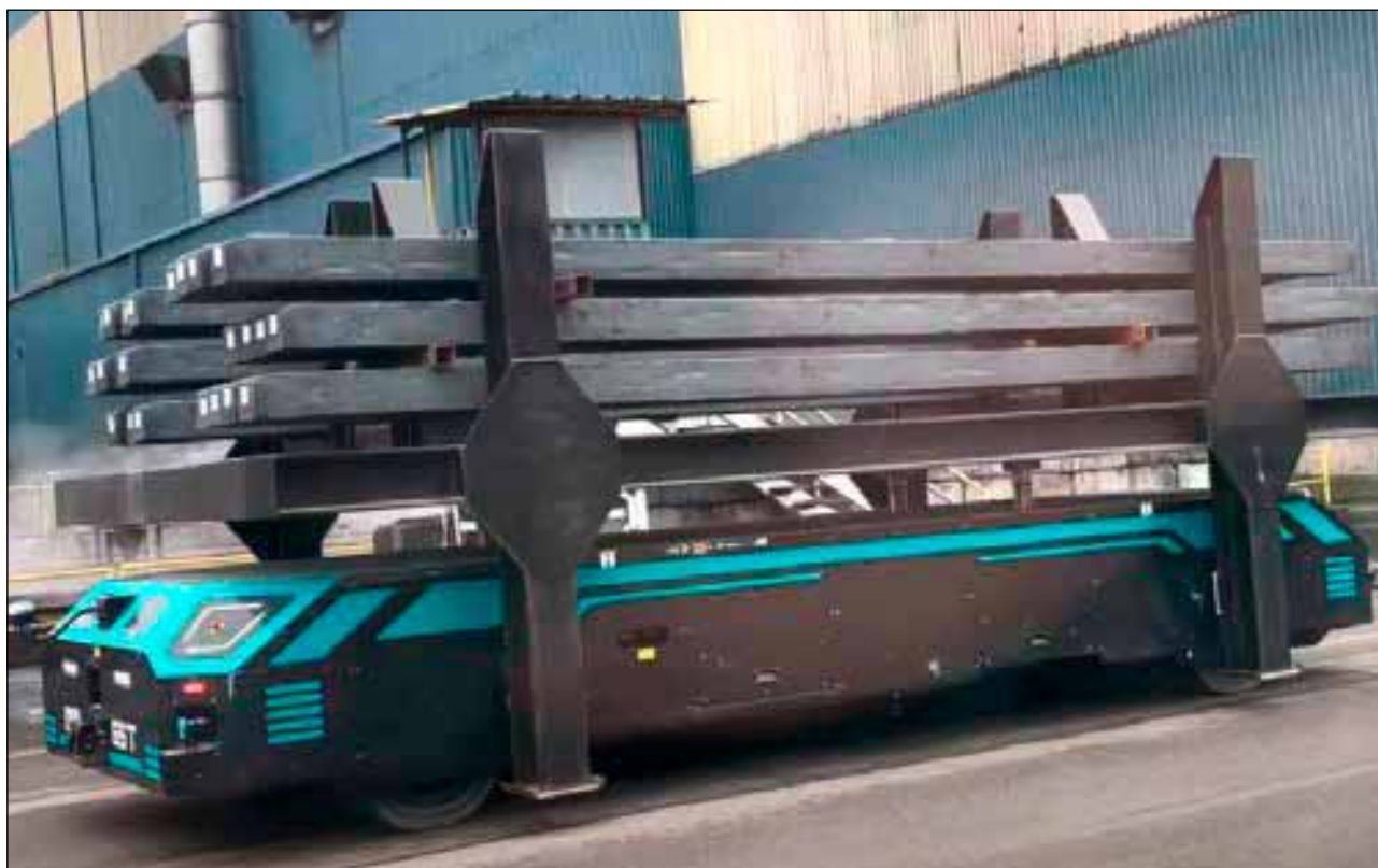
Autonomous guided viche (AGVs), for the transport of Billets at the NAS Factory
